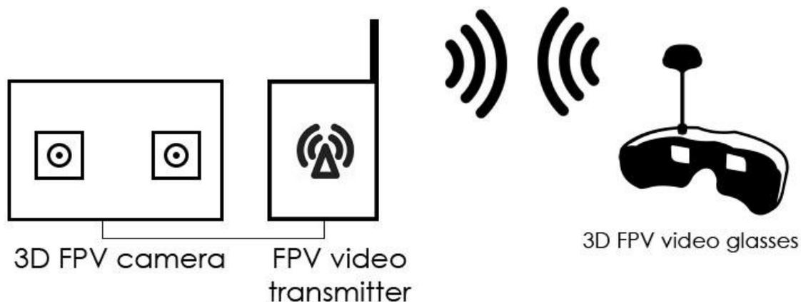
Fig. 3. Video transmission scheme in the FPV system between the camera and FPV glasses
